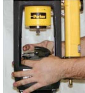
3a. Using a molybdenum disulfide type grease, apply a thin layer of grease to the die bowl.
