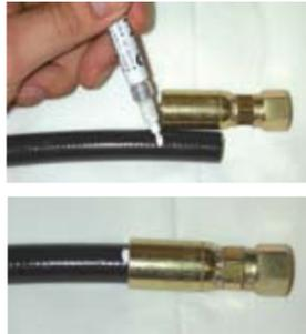
1. Place the hose next to the fitting and align it with the knurl marks on the fitting shell. Mark the length on the hose. Push hose into the fitting until the mark on the hose is even with the end of the fitting shell (lubricate hose\*, if necessary).
