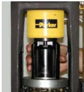
5. Slide pusher into place onto shoulder bolt.
