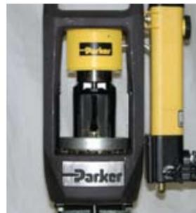
6. Position the hose and fitting in dies from below.
