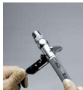
10. Measure crimp diameter of each fitting at the top, middle and bottom of the shell. Take measurements at a minimum of three places around the shell circumference. Verify crimp diameter is within tolerances.
