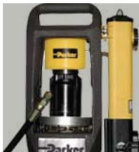
9. Release pressure, remove finished assembly. Check crimp diameter.
