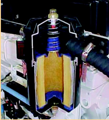
Cummins QSM11 marine engine with CCV cutaway
