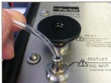
Attach OUTLET (Ø 4mm) hose
