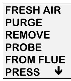
This message indicates that the analyser needs to be reset in fresh air. To do so, ensure that the analyser is in fresh air and press Send / S
